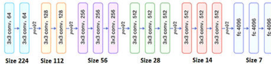
Fig.3. Fundamental Structure of VGG-16
