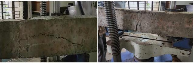
Fig. 4Failure and cracking pattern of beams
