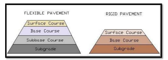
Fig.1- layers of flexible and rigid pavement
