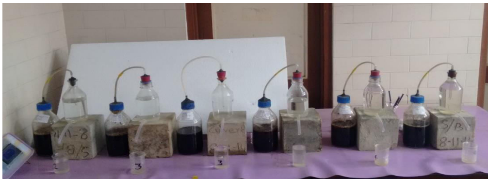
Fig.1 (a) An-aerobic batch reactors setup for various mixing proportions and pH
