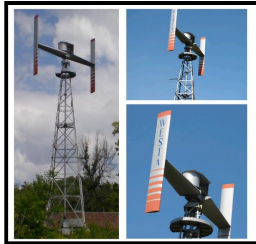
Figure 8. Savonius Rotor combined with Darrieus rotor (Redchyts et. al. 2024)
