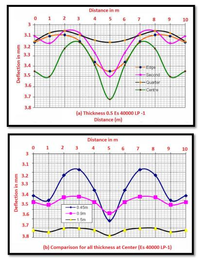
Figure -6, Deflected shapes at Loading pattern -1
