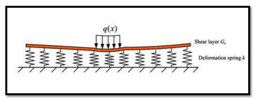
Figure -1, Pasternak foundation Model
