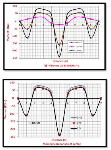
Figure -7, Moment diagram for Loading patten -1
