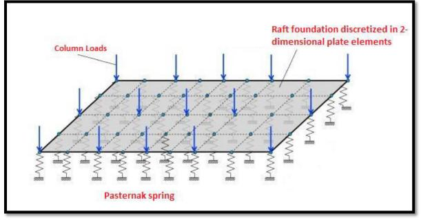
Figure-2, Structural idealisation of raft and supporting soil
