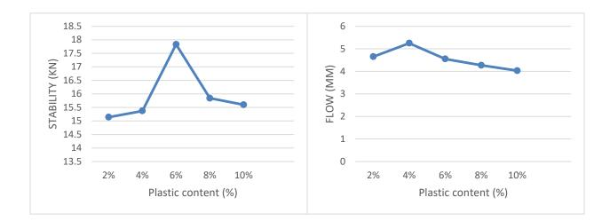
In the experimental study the maximum stability value is 17.83 KN corresponding to the 6% plastic content. So the optimum plastic content is 6%.
